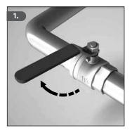
1.Turn the valve handle to the off position.
