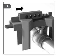
Slide part Y on to part X to connect the two halves of the ball valve lock. The valve handle must be enclosed above, below and at the sides in this case.
