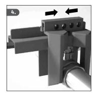
4. Press the two halves together until the valve is tightly enclosed.
