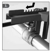
2. Attach part X from above to the valve handle so that the lock tightly encloses the valve body and the valve handle.
